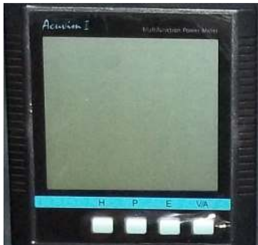
Figure 4. Acuvim II Power Meter
